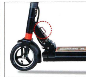
Step 5: Pull out the red lever, and fold the scooter stem at the same time
