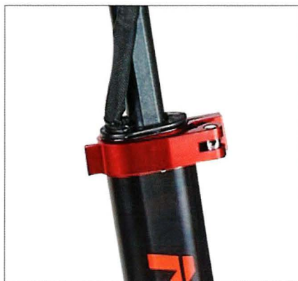
Step4: Fasten the nut and buckle (make sure the stem fixed well)
