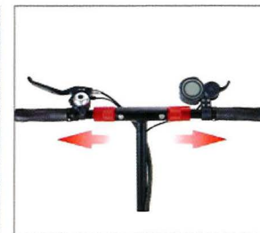
Step 2: Loose the red rods and fold the T handle bar
