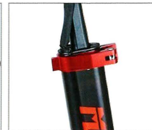
Step 3: unscrew the nut and loose the buckle
