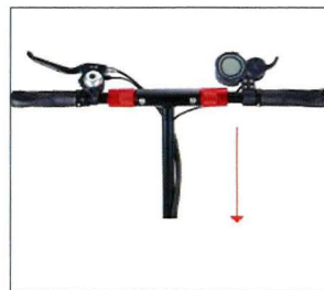
Step 4: Pull downward the T handle bar
